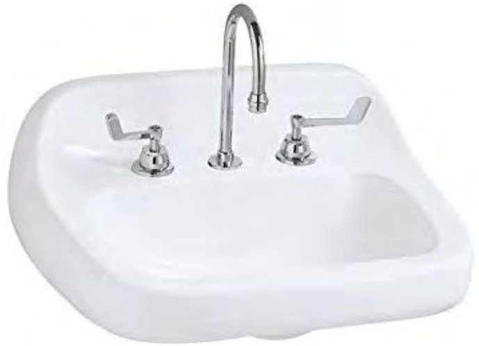
Wall hung lavatory with backsplash, 8” on center holes, gooseneck faucet, wrist blade handles
