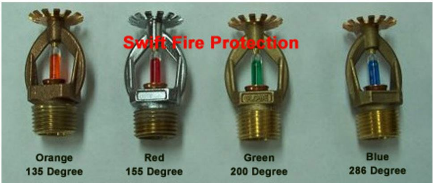
Common contemporary sprinkler head frangible bulb temperature ratings
