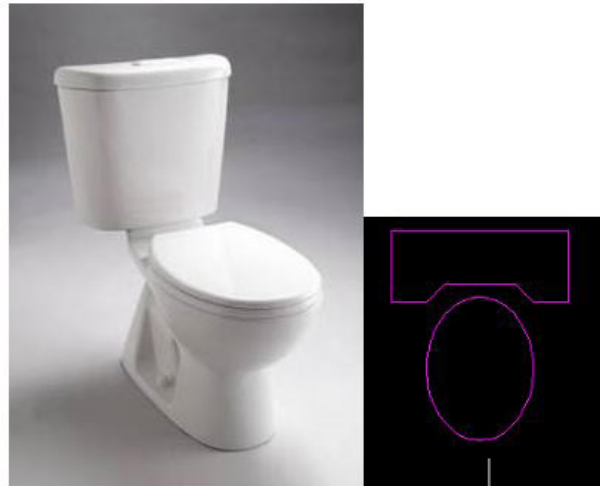
Flush tank floor mount toilet symbol
